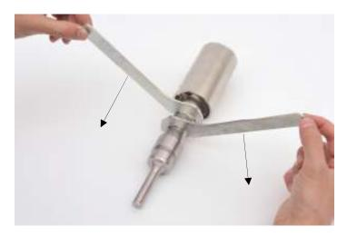
5. The tips on replaceable tip probes can be removed for cleaning and/or replacement. Use alcohol and a cotton swab to remove any debris on the threading of the tip or probe.
