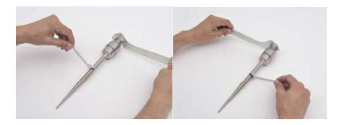
\*Note: When tightening a Microtip the tip must not be in contact with the work surface. Always have the tip extending off of the table or work surface to minimize stress to the tip.
